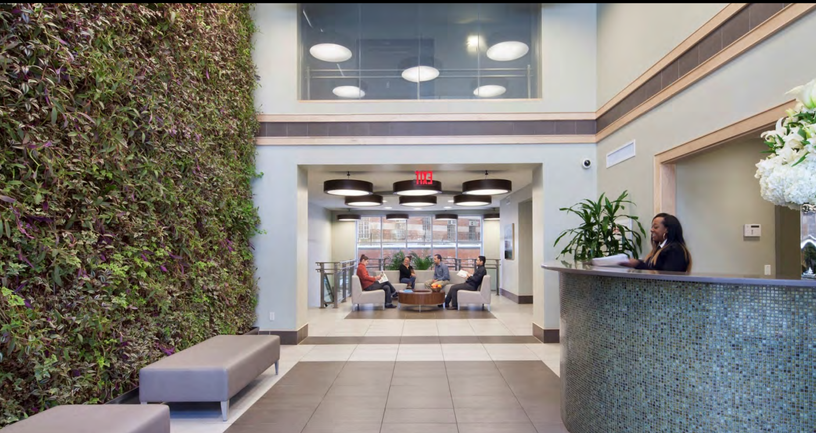
LOBBY GREENWALL: The GreenWall provides a landscape transition from exterior to interior and helps increase indoor air quality. The open stairwell at rear encourages walking, reduces elevator use and electric loads. Tile floors in public areas minimizes maintenance. Interior second-floor glazing allows sunlight into upstairs hallway. Rear lobby glazing (also two-story) allows light into cellar and rear.
