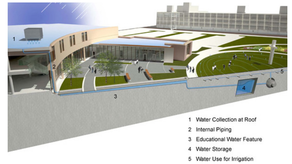
Figure 5 Perspective showing stormwater flow from building roof to cisterns. (Courtesy of Andropogon Associates, Ltd.)
