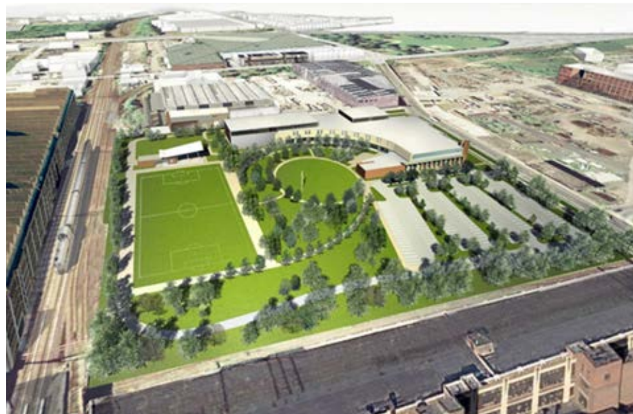
Figure 3 Site plan shows building located in the upper right corner of site leaving approximately 9.4 acres for recreation fields, porous parking and rain gardens. Contaminated material is buried in the area at the lower left corner of the site, between the recreation field and access road/path. (Courtesy of MGA Partners)
