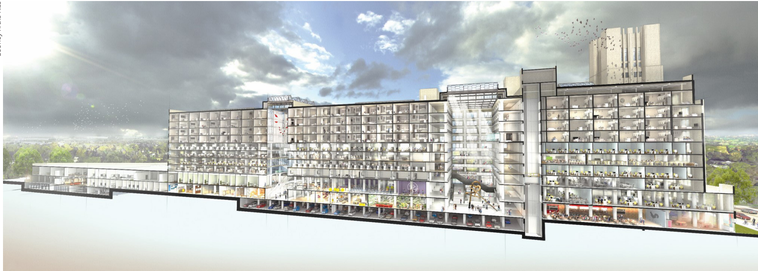
The interior of the building is organized around three new 10-story atria that admit light, connect programmatic elements, and promote a sense of community.
